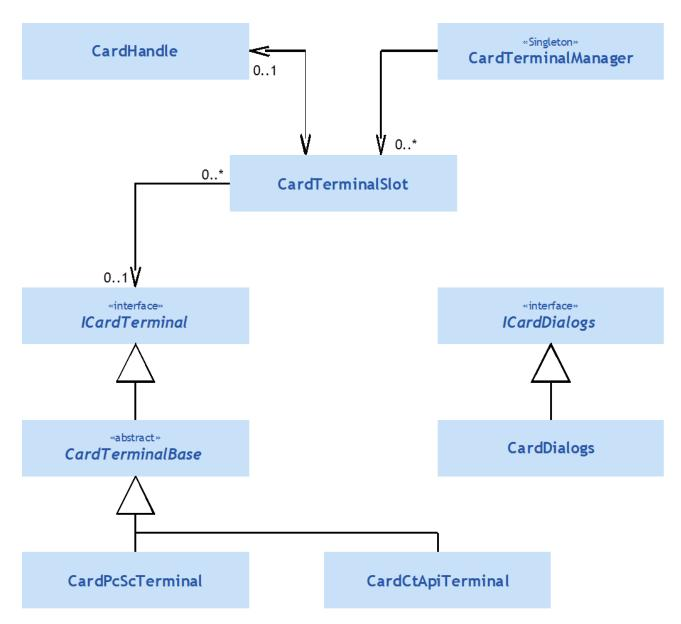
For each card reader slot there is an instance of the class CardTerminalSlot that connects the CardTerminalManager and the CardHandle to the ICardTerminal interface.
